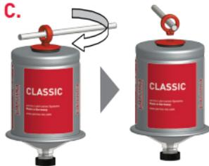
Rotate the activator until the eyelet shears off. **DO NOT** snap the eyelet off by pushing to the side. Use a **ROTATING ACTION ONLY.**
